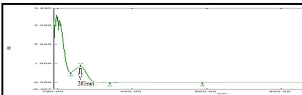
Figure(3.5) Ni(II) –Vitamin C complex in water solution \lambda_{\max}=261\text{nm}
